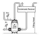
•The discharge capacity is determined by the motive medium, motive medium pressure (P<sub>m</sub>) and back pressure (P<sub>2</sub>).
